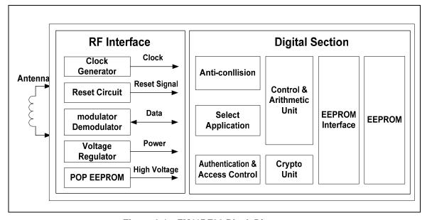
Figure 2-1 FM11RF32 Block Diagram
