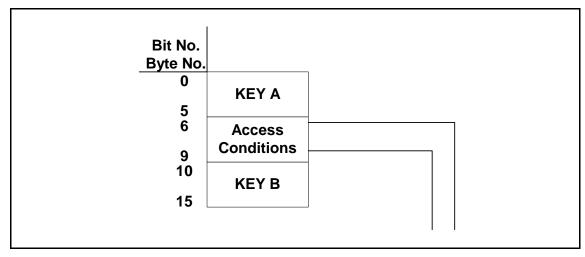
Figure 4-2 FM11RF32 Structure of Block 3
