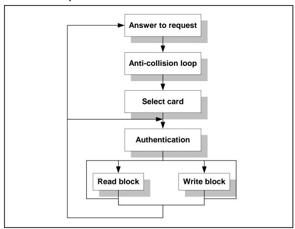
Figure 2-2 FM11RF32 Transaction sequence diagram
